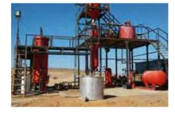
Rapid: The temperature of the desorption electrolysis can reach  $150^{\circ}$ C (30-55 $^{\circ}$ C higher than that of other models at the first stage), and the working pressure of the system can reach 0.5(MPa) (0.2-0.5(MPa) higher than that of other models at the first stage). Therefore, the time for desorption electrolysis is very soon, which is generally 12 hours, with nearly 3 times shortened.
